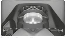
Hydraulic Steering Damper 3 steering positions to quickly control the stifness. It adds riding precision by removing undesired input in rougher conditions. It provides a premium feeling and improved control to the rider.
